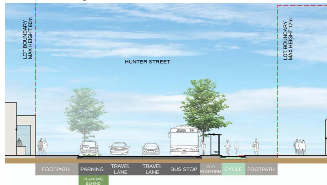
Section 03 - Bus platform at Hunter Street
